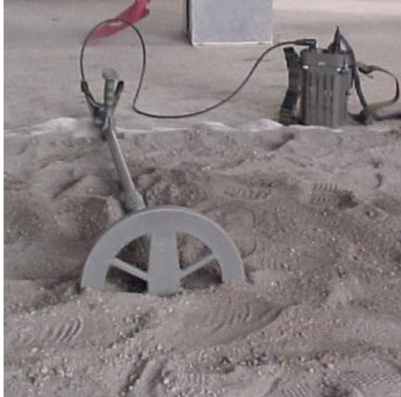
Then take a test-mine (holding it with its top facing the underside of the Search-head) and move it towards the search-head. The person doing this must not wear a wristwatch or metal rings. When the detector starts to signal, make a mark on the ground. Bring it forward again and again making many marks to trace an outline of the area inside which the mine would be found. To get an accurate shape, a mark should be made every two centimetres.
