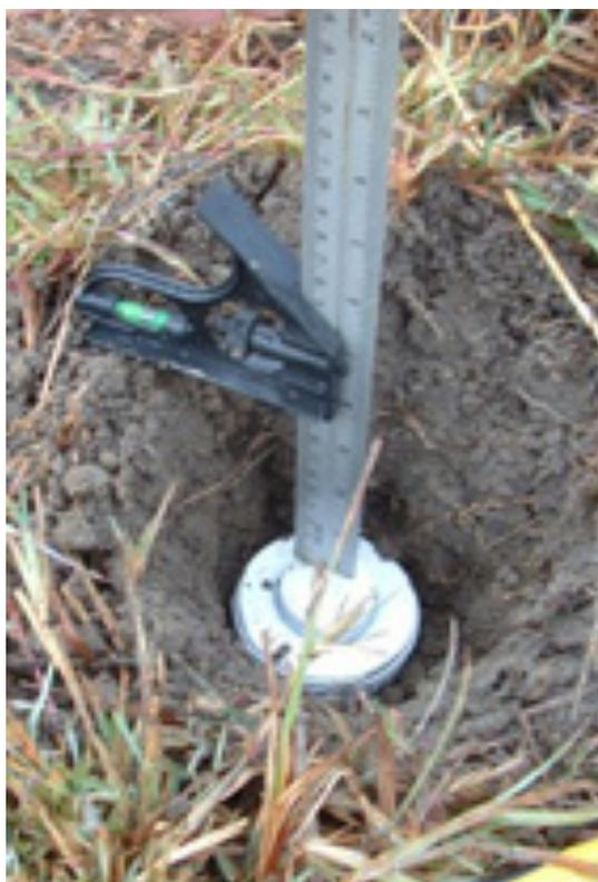
An adjustable set-square like the one shown above can be used to ensure that the target depth is reliably achieved. It is the Task Supervisor's responsibility to ensure that Test areas are metal free before target placement and that target mines are placed at the required depth.
