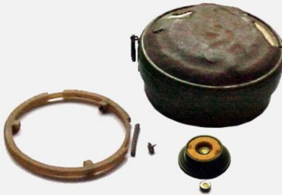
The metal content of a Type 72a is shown above. The white plastic ring is inside the top of the mine and is the sprung loaded arming-ring. The spring is a long, thin coil-spring which is very hard to detect with a metal-detector. The metal content of the mine is so low that it can be impossible to detect with any modern metal-detector when the mine is in electromagnetic soil at a depths of 10-15cm.
