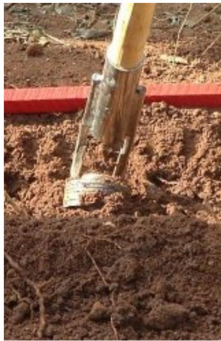
The picture shows a mine being lifted out of the ground by the Harrow-rake. When this occurs, the rake should be withdrawn by reversing it and then lifting it away.
