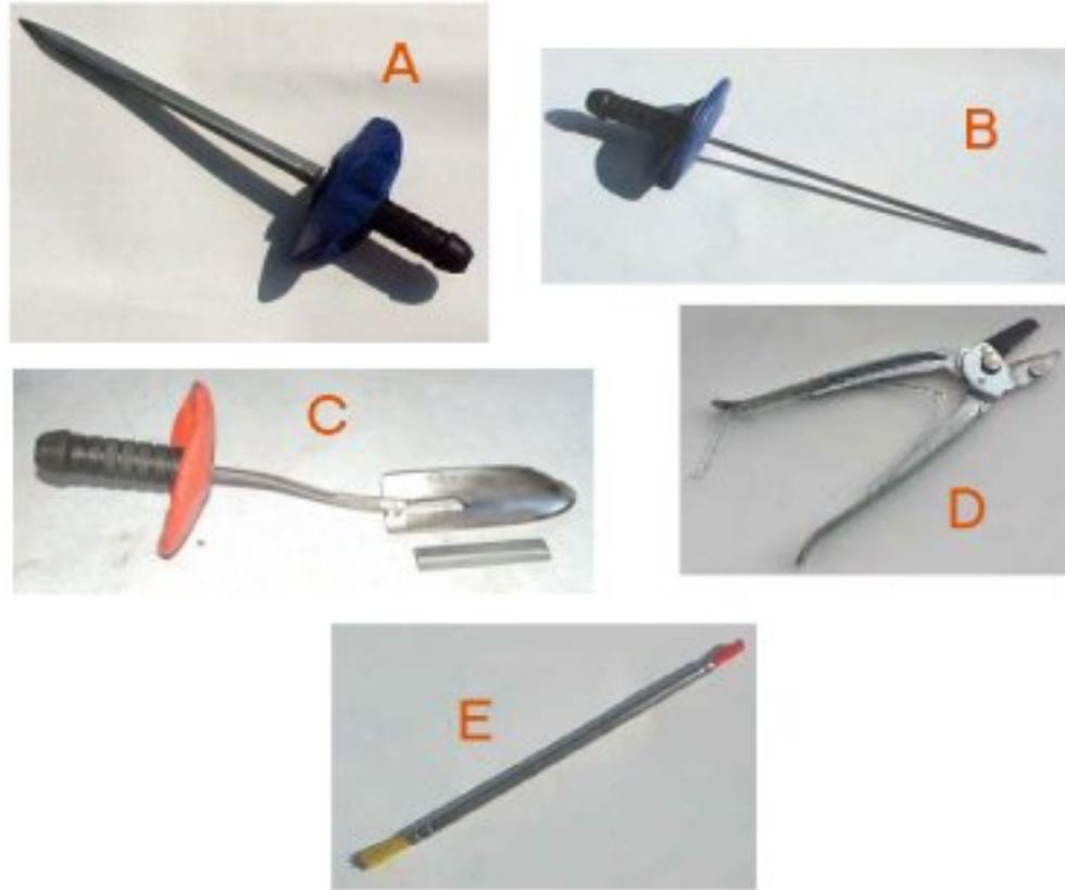
**A:** A [pick-prod](#) designed to be inserted a small way and twisted to break hard ground. A blade may be substituted for this as long as the blade is 30cm or longer.
