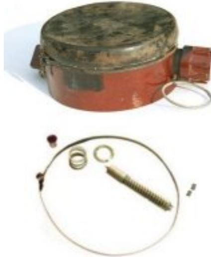
The Chinese Type 58 AP mine is reported to be an identical copy except that attempts to disarm the Chinese mine by unscrewing the booster charge and detonator are reported to have led to initiations.
