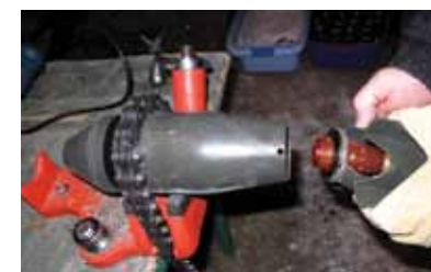
Removing the fuze from a PTAB-2.5.
