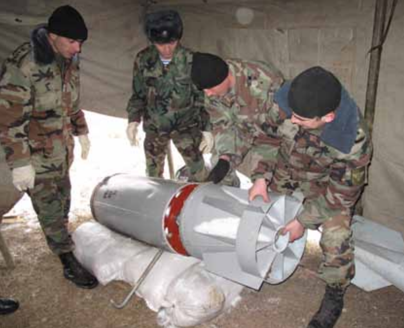
Moldovan soldiers, under supervision, removing the tail from an RBK-500 cluster bomb.
