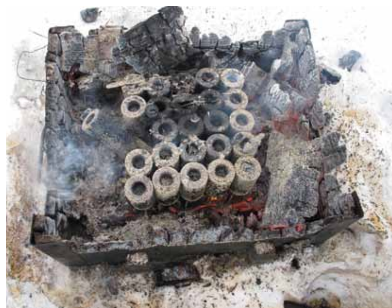
AO-1Sch bomblet bodies after the explosive charge has been burned out.
