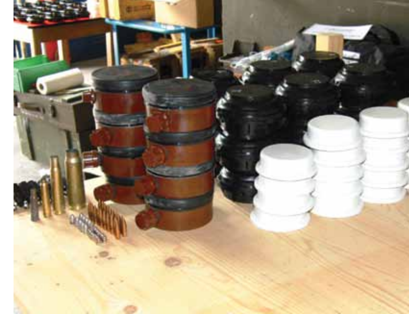
Objects used in the test. From left to right: metal clutter (ammunition belts, cartridges, bullets) and mine-like targets (Gyata-64, PPM-2, ERA calibration target).
