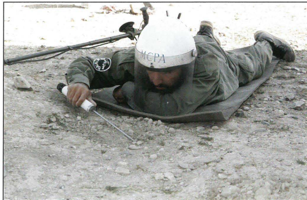
Self-monitoring prodder. Self-contained, no wires.
