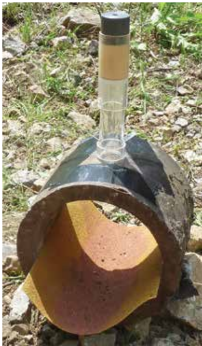
Disruptor being used against an inert target.
