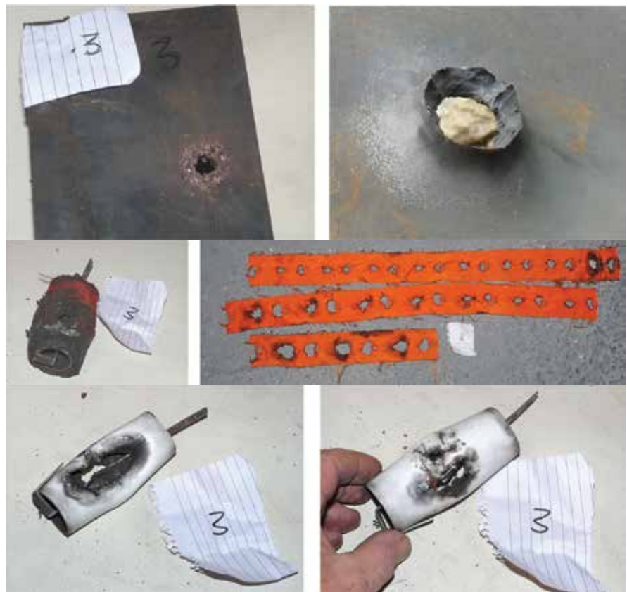
The witness pieces provided a valuable, permanent record of the impact and the spread of material inside the targets.
