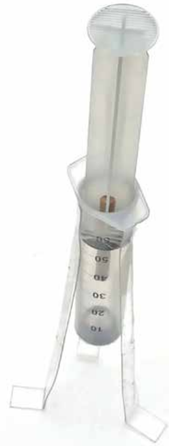
An improvised and low-cost disruptor body with all of the variable control features of those used in our tests.
